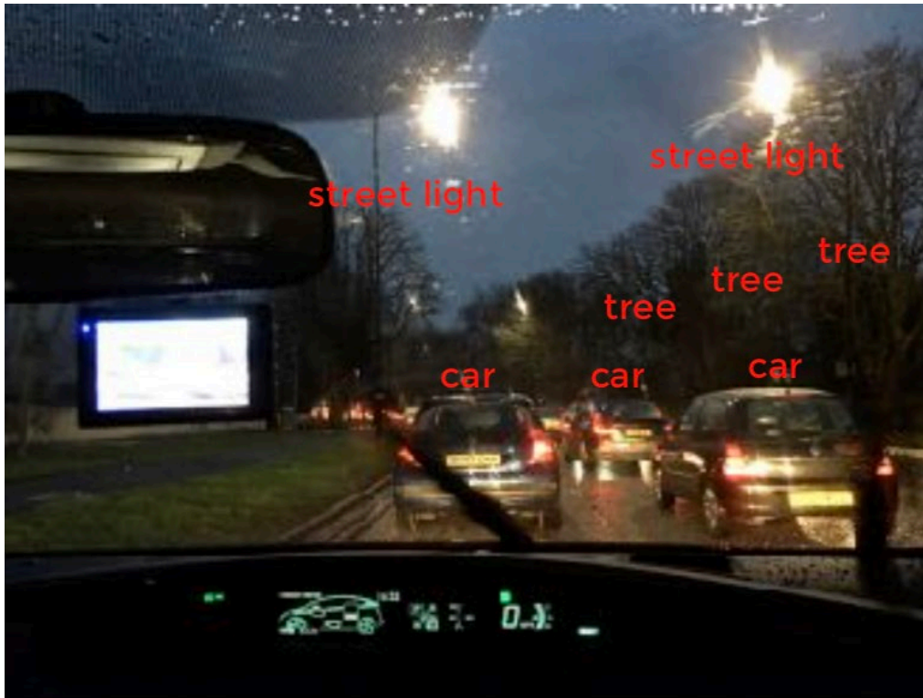
Figure 3: A simplified example of how a car detects objects from image or video. The original photo was taken by Herry Lawford. ( https://www.flickr.com/photos/herry/ ).
